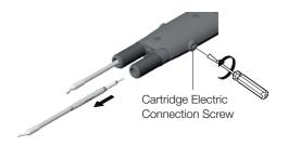
Important: It is esential to insert the cartridge till the end for a good connection.
