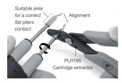
Use a flat pliers in the indicated area for a correct tip alignment.
