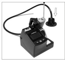
**3** Connect the fume inlet duct for compact stations to the accessory for stand aspiration (Ref. FAE030/FAE040).
