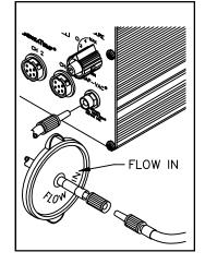
Connect the male fitting of the 137cm (54 inch) length of air hose to the female quick connect hose mount fitting on 2.5cm (1 inch) air hose (connected to VisiFilter) for desoldering, or into the Controllable PRESSURE Port for hot air jet operation.
