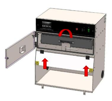
Both filters MUST be fitted when the extractor is in use.
