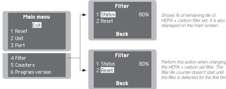
Perform this action when changing the HEPA + carbon set filter. The filter life counter doesn't start until the filter is detected for the first time.
