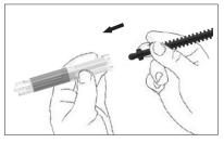
3. Insert the plunger rod in the syringe barrel to eliminate air and press the solder past.
