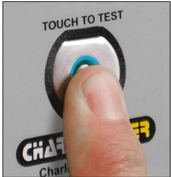
Figure 10. Bridging the test switch's contacts to initiate the test
