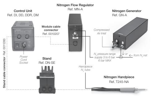
Nitrogen Gas Circuit ----- Electric Circuit
