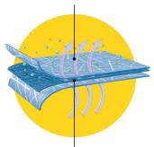
Middle Layers – Intricate web of microfibers that filter out many water-based liquids and dry particulates
