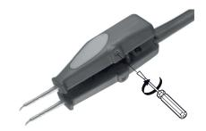
**Important:** Tighten the screw again being careful not to over-tighten. This is necessary for the tool to function.
