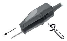
Loosen the screw and remove the cartridge. \!\!\!\!\ Use a flat pliers if still hot.
