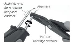
Align the tip of the cartridge. Use a flat pliers in the indicated area for a correct tip alignment.
