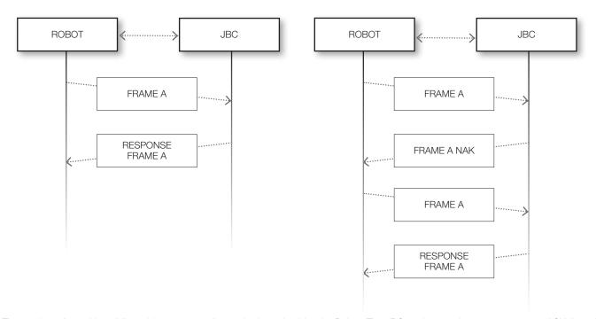
The number of repetitions followed by erroneous frames is determined by the Robot. The JBC equipment does not expects an ACK from the information the Robot sends. If the Robot receives a frame with errors, it can not ask this to be resent, so that it only can repeat everything once again.
