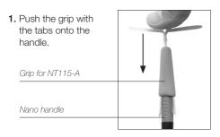
To remove the tabs, hold the grip and pull them out. Use a pliers if necessary.
