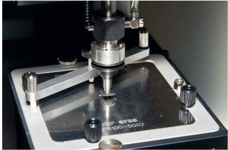
Component is lifted off the print stencil
